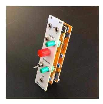
I built this voltage controlled filter for my techno rack. It's based on "Korg late MS20 filter" by René Schmitz.
